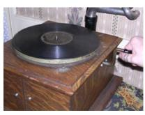
3. Start the motor by swinging the Break Lever toward the cabinet. This will make the table start turning. Wait a minute or two for the wheel to start spinning up to speed.
