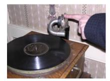
2. Wind the Victrola using the Winding Key.
